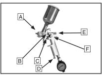
Figure 15. Lubrication points.
